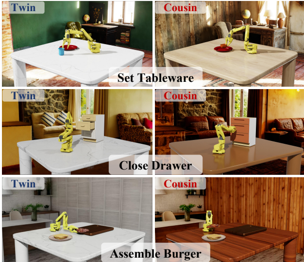
Fig. 10: Additional Simulation Tasks. Visualization of the Digital Twin (left) and generated Digital Cousin (right) environments for the tasks not displayed in the main manuscript.
