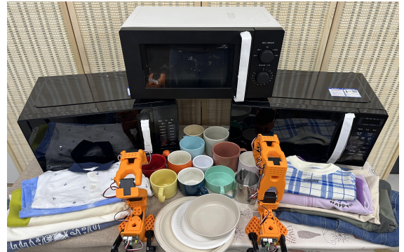
Fig. 4: Real-World Setup. The hardware configuration consists of two lerobot arms and diverse object instances.
